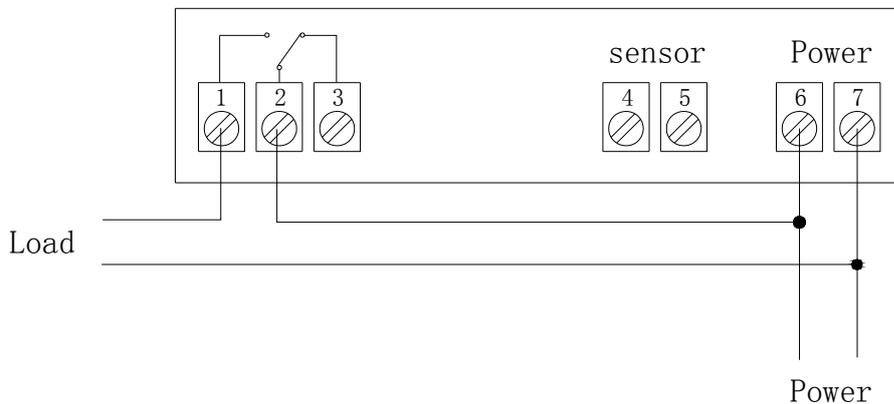
Terminals 1 and 2: Normally opened contact of relay
