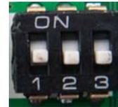
A . Unlocking time is 1 second (default value, all switch is on the below)
